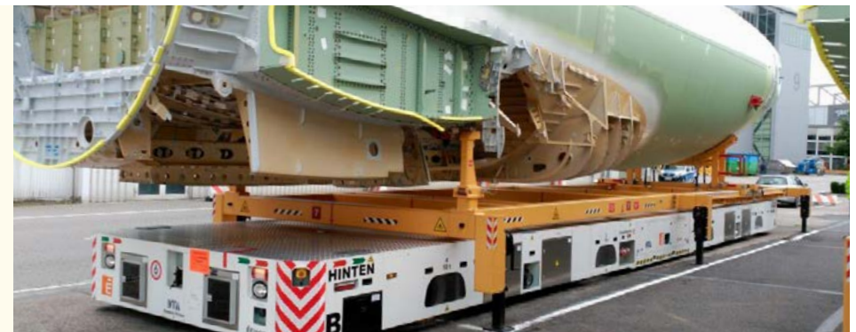
DTA's Dolphin AGVs are fully customizable and capable of carrying a wide range of payloads, such as aircraft fuselages.
