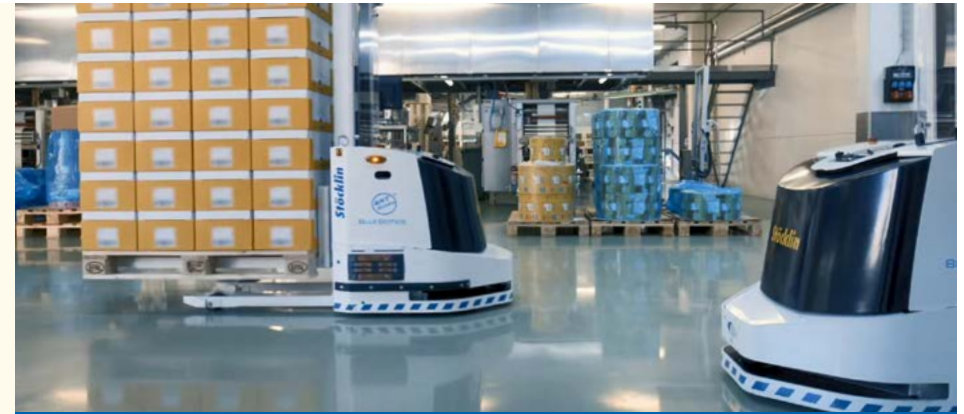
Forked AGVs by Stöcklin Logistik hard at work in a Swiss manufacturing facility.
