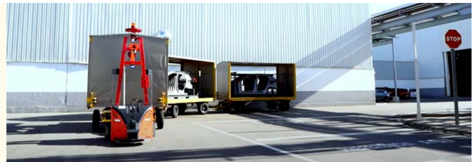
A TriBOT tow tractor by ASTI Mobile Robotics moving several car chassis between facilities.
