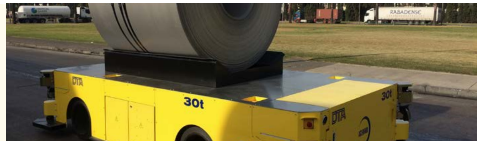
AGVs by DTA transport materials between buildings at a steelworks in Spain.
