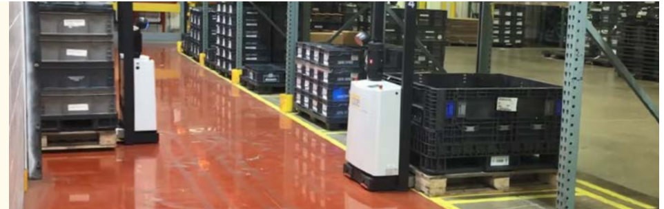
Nipper pallet truck AGVs by F3-Design at work in a U.S. warehouse.
