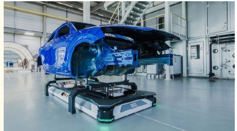
AGVs are common in automotive production, such as this Durr EcoProFleet vehicle , a solution designed exclusively to operate in paint shops.
